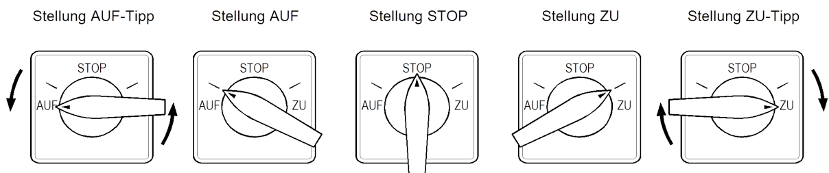
Figure 3: control switch S31
